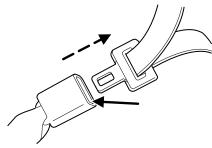
All restraints in the vehicle are combination lap and shoulder belts. While you are fastened in the seat belt, the combination lap/shoulder belt adjusts to your movement. However, if you brake hard, turn hard, or if your vehicle receives an impact of 5 mph (8 km/h) or more, the safety belt will become locked and help reduce your forward movement.
